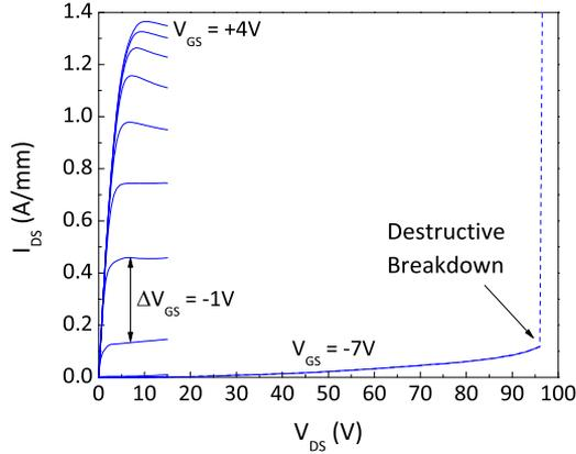
FIG. 2. (Color online) Drain characteristics of the Ta<sub>2</sub>O<sub>5</sub>/AlN/GaN HEMT (destructive breakdown occurs at 96 V for V<sub>GS</sub>=-7 V).
